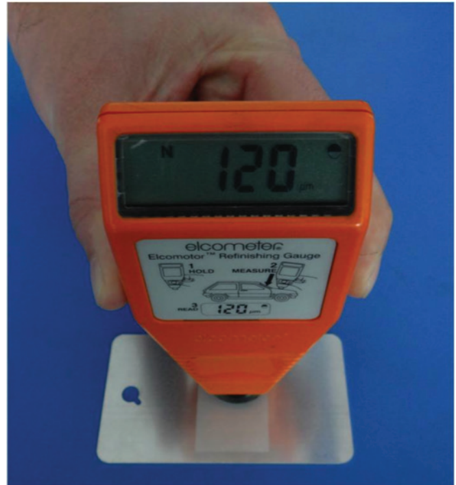
Figure 4. Calibration of the UMD before OP layer thickness measurement
